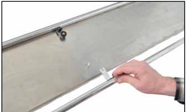
Figure 11 - Remove Brackets and Tubes From the SEP
