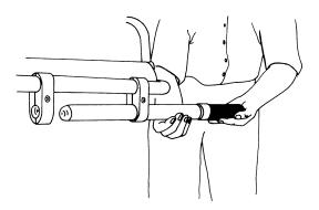
Locate the squad handle in the desired position, then tighten the mount casting bolts. Properly installed, the handle assembly should be clamped tightly, should not rotate or slide on the cot/stretcher frame tube, and the telescoping handle should slide in and out smoothly.
