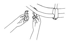
Slide the telescoping squad handle assembly into the mount castings. Properly installed, the handle tube will pass completely through both castings which will be spaced 4-12 inches apart.
