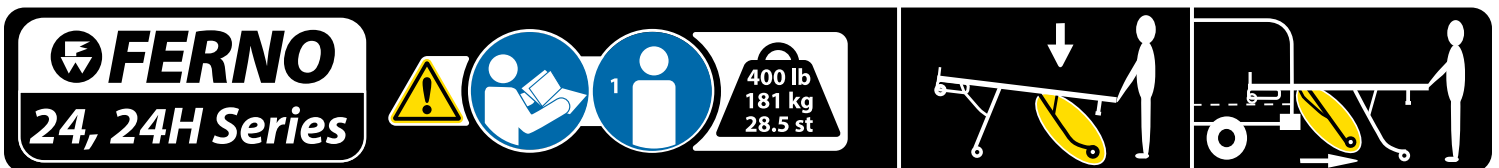
Operator-end Label: Identifies the cot, provides safety and load capacity information, and identifies the function of the control-end control handle.
