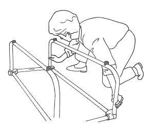
Install the two top braces between the side rails as shown and tighten securely with the four 1 3/4" round head bolts supplied.
