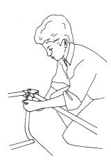
Install the 5" caster assemblies by inserting the stem pin of each caster into the holes on the bottom side of the corner castings, making sure the holes in the stem pin line up with the tapped holes in the corner castings. Fasten the caster assemblies to the corner castings with the 1/2" socket head cap screws and tighten securely.
