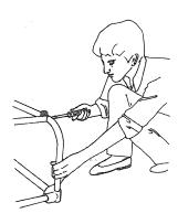
Turn the showroom truck over so that it rests on its rubber bumpers. Fasten the sideralls to the lower frame assembly by inserting a 1/2" socket head cap screw into the tapped hole in each corner casting and tightening securely.
