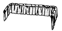
Join the two frame halves by inserting the splice into the frame ends.
